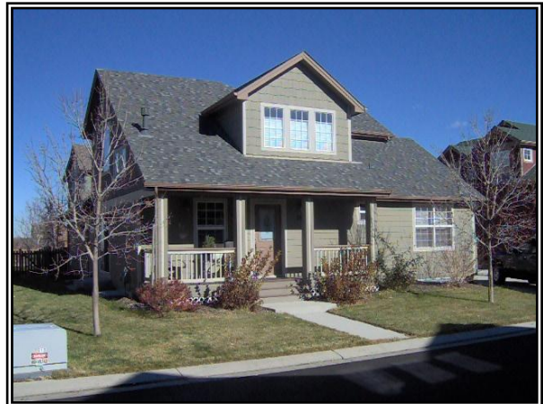
Contemporary Craftsman-style home - Note: expansive porch; street orientation; customized door; window treatment; and dormer.
